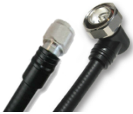
1/2" Flexible (LDF4-50A) 7/16 DIN Male Right Angle to 4.3-10 Male Low PIM Jumper | 123-1DMRHM |123e.com Part Number: 123-1DMRHM-XX-P
